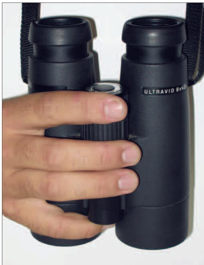
At about 6 inches in length, and weighing in at only 27.8 ounces, the Ultravids are smaller and lighter than most other top-of-the-line full-size binoculars. They comfortably fit both my hand and face. © Derek Lovitch.
