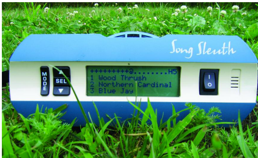
The “Song Sleuth: Audio Birdsong Detective” hears a bird’s song, digitizes it, analyzes it using algorithms, and produces three ranked choices of the singer’s identity. © Derek Lovitch.
